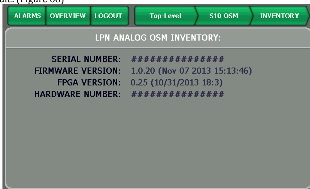
Figure 68 - LPN Analog Module Inventory Screen
