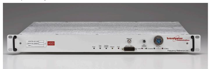
The FRU is a state of the art, high-precision frequency standard capable of outputting ten isolated precision 10MHz frequency reference outputs. The FRU uses an internal GPS receiver to control a precision oscillator with accuracy up to 1 x 10-12 and excellent short term stability
