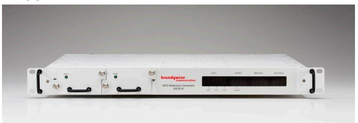
The GPS Time Distribution System (ENTA-R) is a high-availability time-distribution qualified for shipboard use. It receives time from two external GPS receivers as 1PPS and Have Quick, and it uses this over-determined time solution to both remove a faulty input reference and disciplines an internal time base oscillator. The internal time base is used to re-generate multiple 1PPS and Have Quick signals to support other systems.
